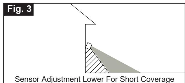
Sensor Adjustment Lower For Short Coverage
