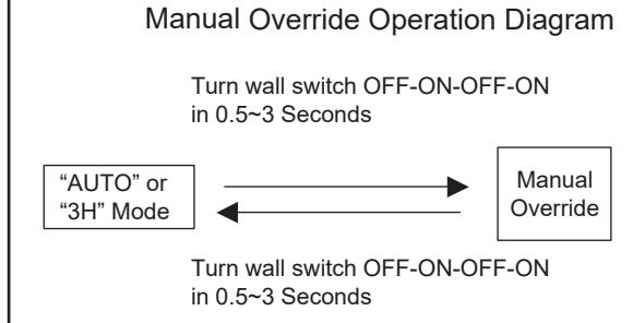
**Note: To make sure the above functions operate properly, always keep the wall switch in the ON position (including the daytime).**
