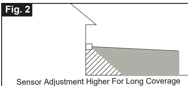
Sensor Adjustment Higher For Long Coverage
