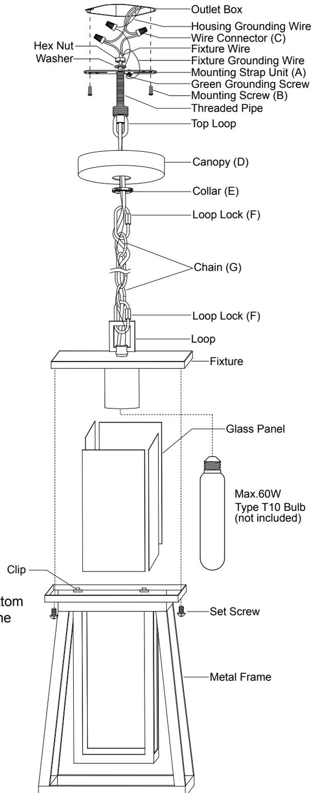
7. Attach the metal frame back to the fixture by aligning holes, secure them with the two set screws.
