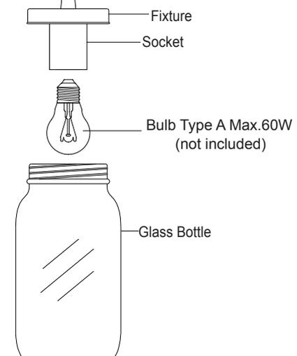
9. Install a bulb(not included). See relamping label at socket area or packaging for maximum allowed wattage.
