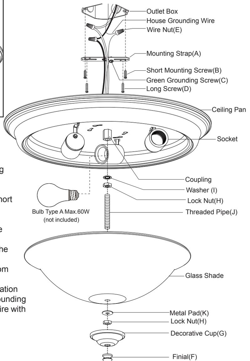
4. Attach the ceiling pan to the mounting strap by inserting two long screw heads into the key holes, and then rotate the ceiling pan until it locks in place, finally secure the screws tightly. (See Fig.1)
