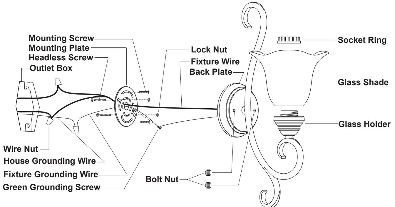
1. Thread two headless screws to the mounting plate, and secure them with four lock nuts (two on each side of the mounting plate). Adjust the length of the headless screws if necessary.
